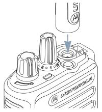
To remove the antenna, turn the antenna counterclockwise.
