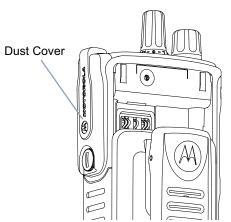
Insert the hooked end of the cover into the slots above the universal connector. Press downward on the cover to seat the lower tab properly into the RF connector.
