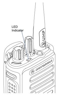
**Blinking green** – Radio is receiving a non-privacy-enabled call or data, or detecting activity or retrieving Over-the-Air Programming transmissions over the air.
