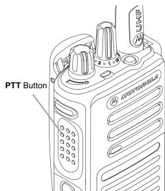
While a call is not in progress, the PTT button is used to make a new call (see Making a Radio Call on page 18).
